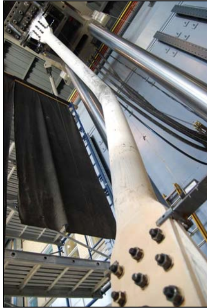
Caption: Full-scale seismic testing of a brace equipped with Cast ConneX™ High-Strength Connectors at the structural laboratories of École Polytechnique de Montréal. The brace pictured is experiencing out-of-plane inelastic buckling, as would occur during a design level seismic event.
